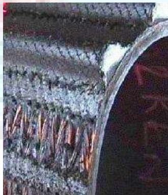
Figure 2 – Breakage failure on belt
