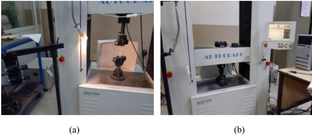
Fig.3. Mechanical Tests, (a) Tensile, (b) Three Point Bending.
